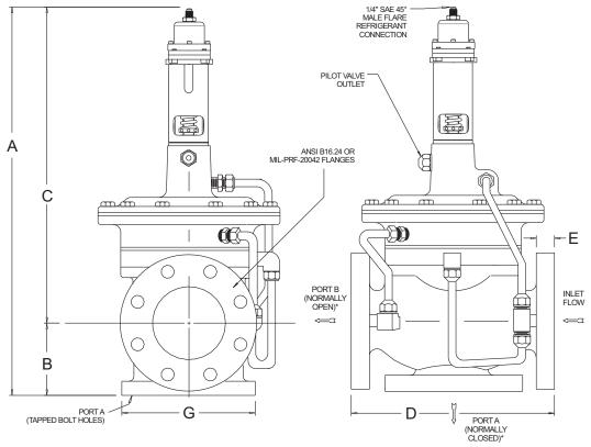
\*NOTE: Normally closed valves open on pressure increase, normally open valves close on pressure increase.
