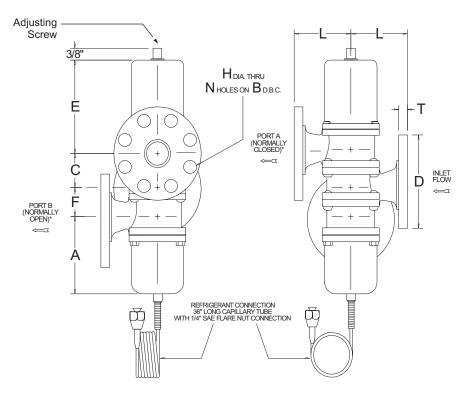
\*NOTE: Normally closed valves open on pressure increase, Normally open valves close on pressure increase.
