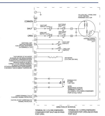
The purpose of the heater as shown in the wiring diagram is to prevent condensation from forming in the actuator housing. Heater is rated at 25 watts. Connect 115 VAC across terminals #7 & #8 to maintain internal actuator temperature at approximately 10°F above ambient temperature.
